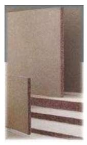
Figure 1 sample of fiber panel boards from herbaceous biomass.
